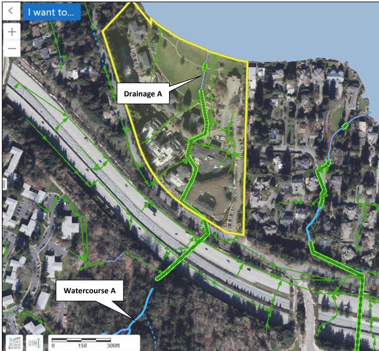
Figure 4: GIS Portal watercourse and stormwater mapping showing Watercourse A flowing north into Drainage A. Note extensive drainage network conveyed into the piped sections above Drainage A.
